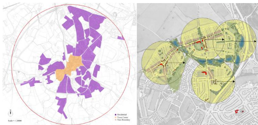
Image of dispersed pattern of an Irish Town and one for the design of walkable routes.
